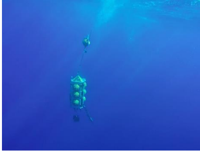
The Edokko Mark I, an unmanned device for capturing images and videos in the deep sea that the Japanese government is testing to help in monitoring mining activities. Image courtesy of JAMSTEC.
